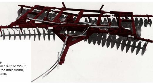
**Series VI ... 30'' Wing Frame.** Available in cutting widths from 18'-3" to 22'-8", Dual wheels are standard on the main frame, with single wheels on wing frame.
