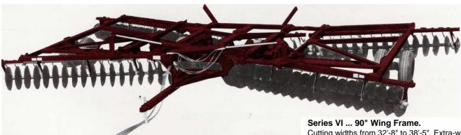
Cutting widths from 32'-8" to 38'-5". Extra-wide wing frames fully support these increased gang widths. Dual wheels standard on both main frame and wing frames.
