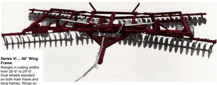
the 60-inch and 90-inch wing frame models fold in 20° from vertical. Transport width is 15'-4".
